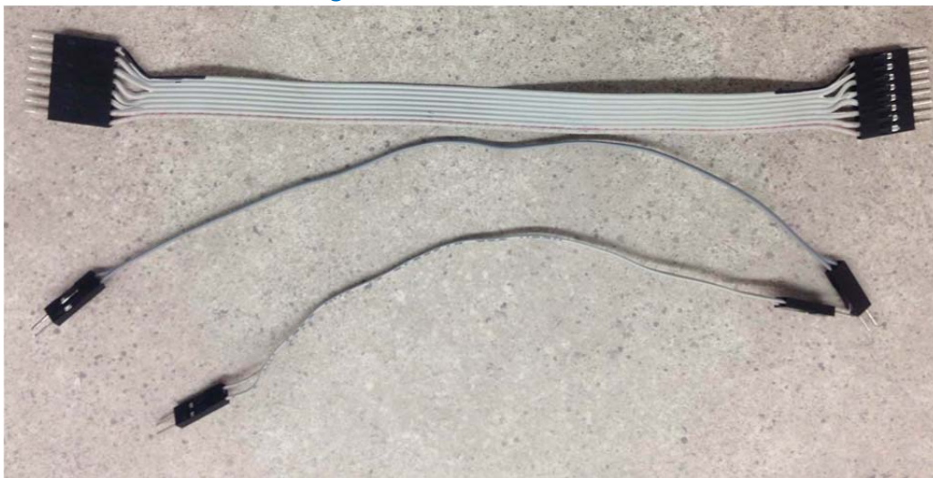
Photo1. Testing Wires: The 8 and 2 leads ribbon cables
